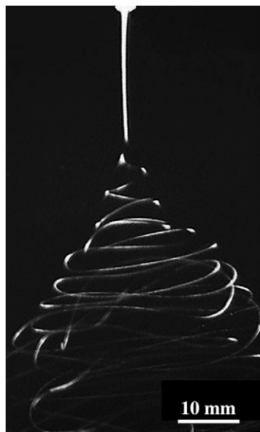
Fig. 3. A snapshot of an electrospinning jet with well-developed loops appearing after the onset of the electrical bending instability at some distance from the nozzle. Some short segments of the continuous jet were not illuminated, and therefore are not seen.
